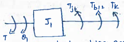
Fig 2: Free body diagram of mass with moment of inertia J_1 .
