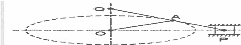
Fig. 9.7. Modified Scott-Russel mechanism.
