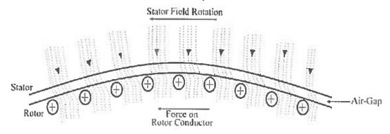
• When the stator winding is connected to a balanced three phase supply, a rotating magnetic field (RMF) is setup which rotates around the stator at synchronous speed (N<sub>3</sub>). Where,
