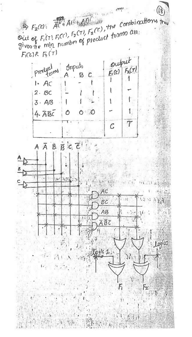
PLA PAL 1. OR array is 1. Both AND& OR fixed & AND array are program array is program. -mable. -mable 2. Cheaper & 2. Costliest & more simpler. complex than PALS, PROM'S. 3. AND array can 3. AND array can be programmed be programmed to to get desired get desired minterns 4. Any boolean g. Any boolean function in SOP function in SOP form cam be form can be implemented using implemented using \$ PAL. PLA.
