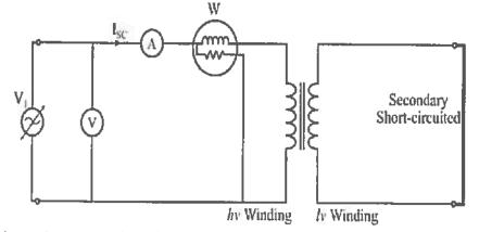
The low voltage source is applied across the secondary winding, which is approximately 5 to 10% of the normal rated voltage. The flux is set up in the core of the transformer. The magnitude of the flux is small as compared to the normal flux.
