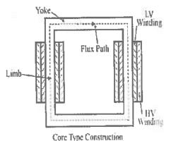
The laminations of the core type transformer are of U-I shape as shown in the figure.
