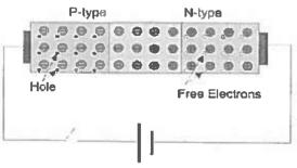
accumulate on the n-side and p-side respectively. This region so formed is called as depletion region. Due to the presence of these positive and negative ions a static electric field called as "barrier potential" is created across the p-n junction of the diode.
