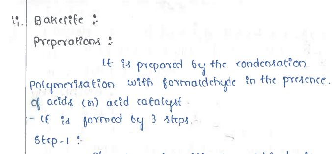
phenol reacts with formaldehyde in the presence of acid to form ortho mono methylol phenol & para mono methylol phenol.
