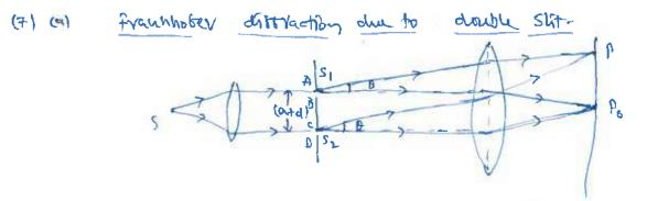
AB and CD are two stits separated by a distance 'd' of each slit width 'a'.
