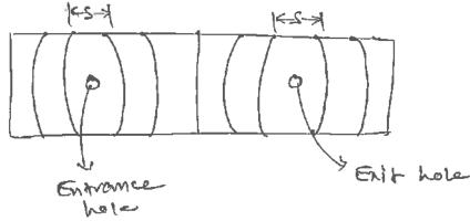
from the figure, the angle O corresponding to a particulow pair of once is related to the distance is blu the arcs
