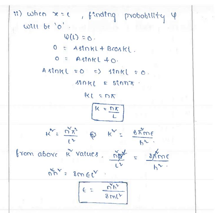
from the above formula, we can calculate energy and this energy in one-dimensional is quantised n = 1 i  $E_1 = \frac{(3)h^2}{8mL^2} = x$ . n = 3,  $E_2 = \frac{(3)h^2}{8mL^2} = 4x$ . n = 3,  $E_3 = \frac{(3)h^2}{8mL^2} = 9x$ . ware function inside a Box 🍃
