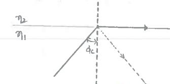
> For the angles of incidence greater than the oritical angle the light is reflected block into the originating dietectric medium and the process is known as total internal reflection.
