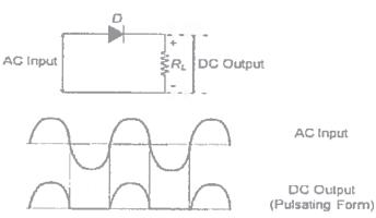
pulses only. The polarity of the output voltage so obtained (across  $R_L$ ) depends on the direction of the diode used in the circuit of half-wave rectifier.
