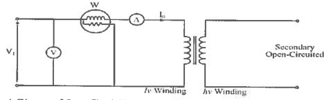
Circuit Diagram of Open Circuit Test on Transformer
