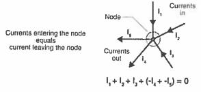
In the above figure, the currents I1, I2 and I3 entering the node is considered positive, likewise, the currents I4 and 15 exiting the nodes is considered negative in values. This can be expressed in the form of an equation:
