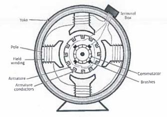
Figure : constructional details of a simple 4-pole DC machine. The above figure shows constructional details of a simple 4-pole DC machine. A DC machine consists of two basic parts; stator and rotor. Basic constructional parts of a DC machine are described below.
