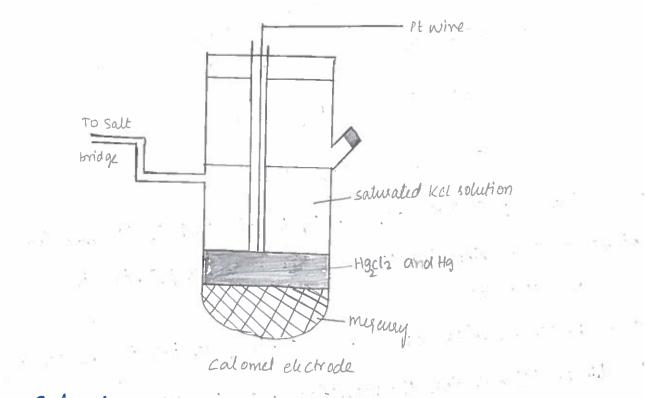
Calomel electrode is a metal-metal salt ion electrode. It consists of mercury, mercurous chloride and a solution of kcl. Mercury is placed at the bottom of a glass type having a side type on each side. Mercury is covered by a parte of mercuroous chloride (calomel) with mercury & Kcl
