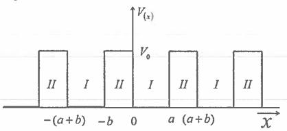
The Schrödinger wave equation for an electron moving in one dimensional periodic potential is
