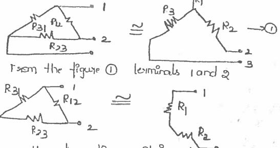
From the above figure it is observed that Riz and Pzi connected in Servies and that combration in parallel with Riz - In star correction Ri and Ri ave connected in services.
