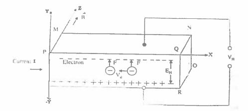
On the other hand, the loss of electrons from the upper of the material becomes positively charged. Hence potential  $V_h$  called Hall Voltage appears between the upper and lower surfaces of the semiconductor which establishes an electric field Eh called the Hall electric field. The electric field  $E_H$  exerts an upward force  $F_h$  in the electron is given by
