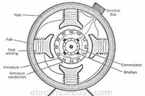
to them. Pole shoes serve two purposes; (i) they support field coils and (ii) spread out the flux in air gap uniformly.
