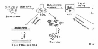
Fig: Schematic representation of Sol-Gel process for synthesis
