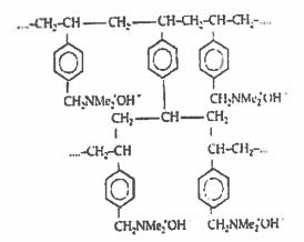
N-methyl ammonium hydroxyl styrene co-polymer -anionic resin
